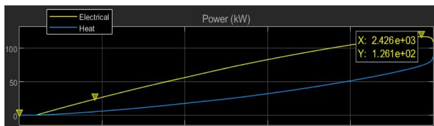
Fig. 7. : The thermal and electrical power obtained from the fuel cell after optimization
