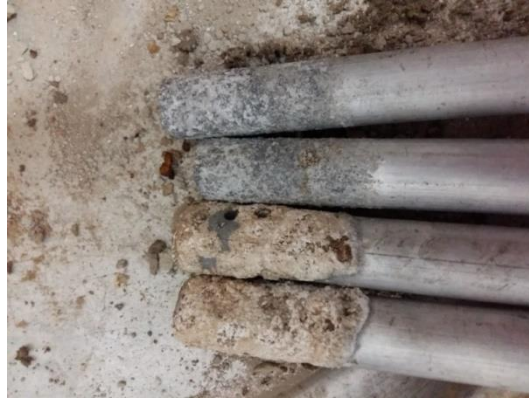
Figure 7: Formation of Oxide Layer on Aluminum Electrodes in a 3-Day Period
