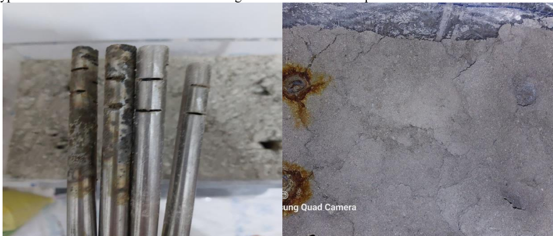
Figure 6: High corrosion of iron electrodes against water and minerals in the soil
