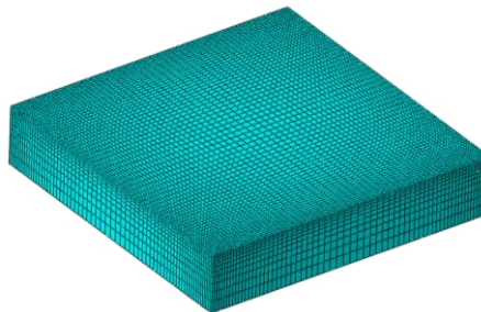
Figure 10. Foundation meshing of the structure.
