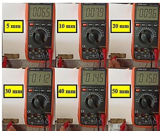
Figure 3. Surface resistance of the Pt electrode along the length of the IPMC
