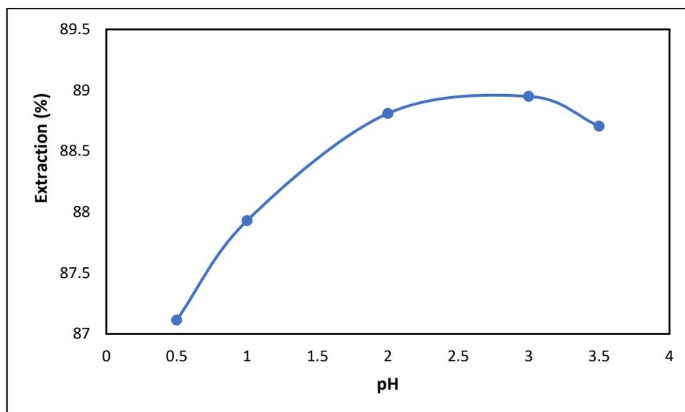
**Fig. 1.** Effect of pH on Cu(II) extraction (Surfactant Concentration= 1 V/V%, Mixing Speed= 0 rpm)
