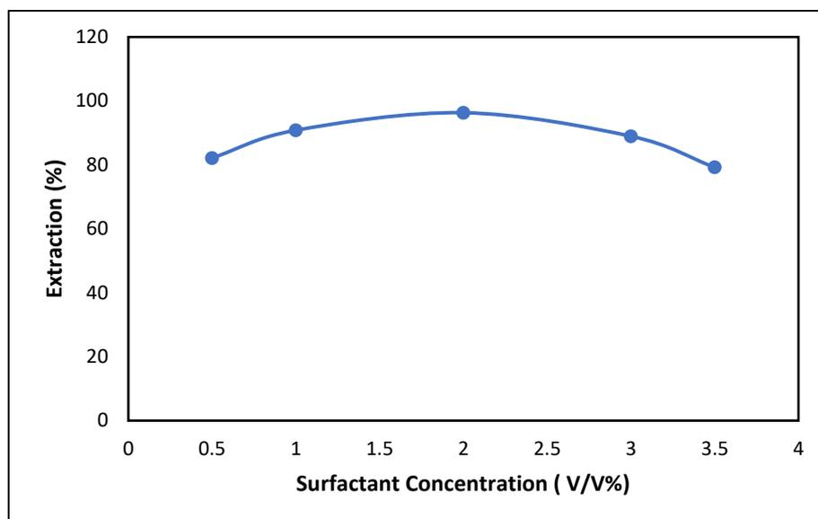
**Fig. 2.** Effect of surfactant on Cu(II) extraction ( $pH=1$ , mixing speed= 0 rpm).
