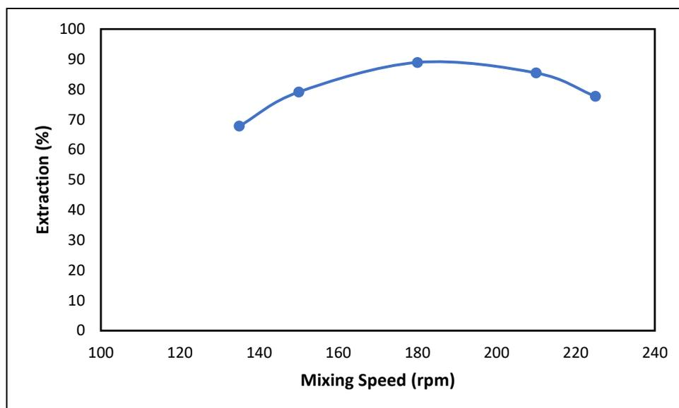
**Fig. 3.** Effect of mixing speed on Cu(II) extraction (Surfactant Concentration=1 V/V%, pH=1)
