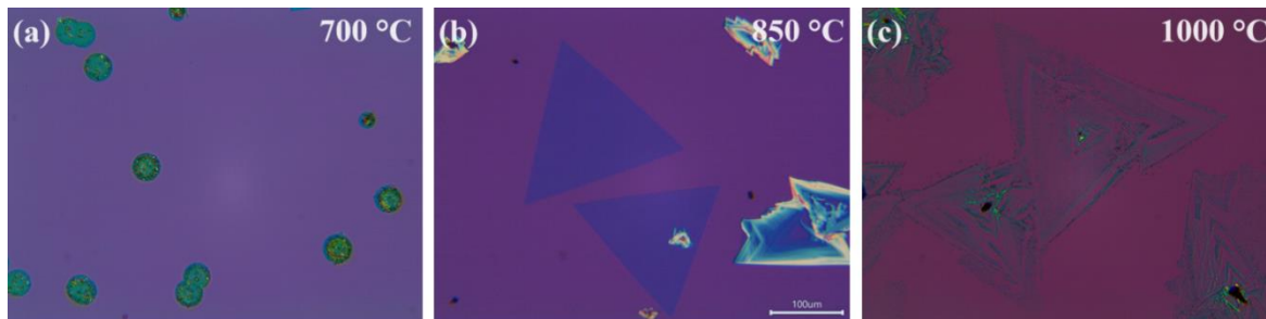
Figure 3. Optical Microscopy images of \text{WS}_2 samples grown on \text{SiO}_2/\text{Si} substrate at a. 700 °C; b. 850 °C and c. 1000 °C growth temperature.
