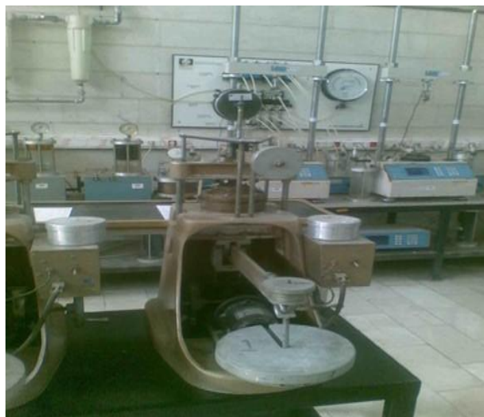
Fig 4 – One-Dimensional Consolidation Test Apparatus
