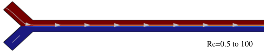
Fig. 3. Concentration profile of a simple y-type micromixer in the range of Reynolds numbers from 0.5 to 100.
