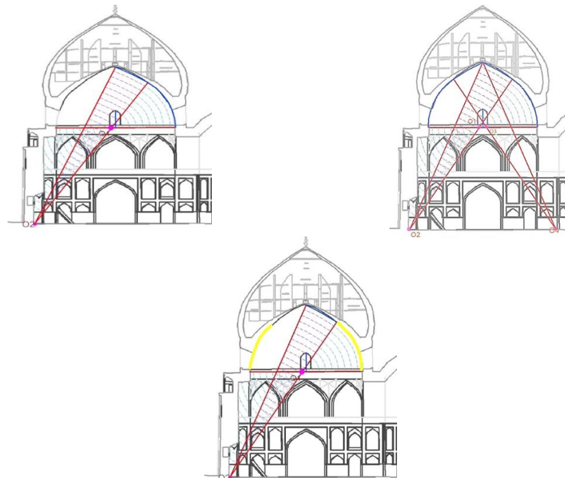
Fig. 14. Investigation of the type of arch in the dome of Shah Mosque in Isfahan [27].
