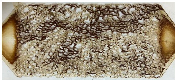
Fig 5. oil displacement of the nanofluid with 250 ppm \text{SiO}_2 and 1000 ppm \text{Al}_2\text{O}_3 in 70^\circ\text{C} .
